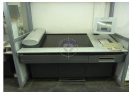
Prinect Image Control is a color measurement system for regulating the ink zones of the printing press
